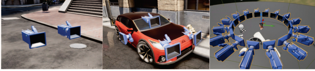
Figure 2. UnrealStereo is a synchronized multiple camera system. From left to right are a two-camera system used in our stereo experiment, cameras mounted on a virtual car and a 16 camera system surrounding a virtual human head.
