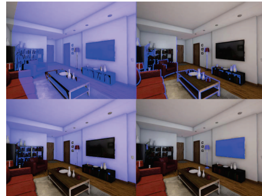
Figure 5. Binary masks that we compute from object mask and material property. From top left in clockwise are: mask for non-occluded region, object boundary region, specular region and textureless region. Best seen in color.
