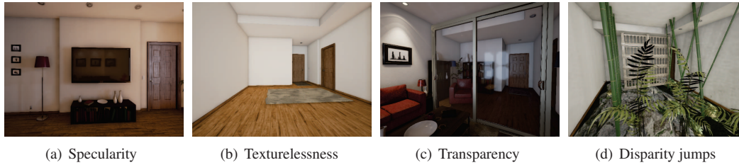
Figure 4. From (a) to (d) are cases we designed to test algorithms. They are specularity, lack of texture, transparency and disparity jump. In (a), the screen of a TV is set to be specular. In (b), the wall and the ceiling in the room are made textureless. In (c), the sliding door has a transparent surface. In (d), objects such as bamboos, fences and plants give frequent disparity discontinuities.
